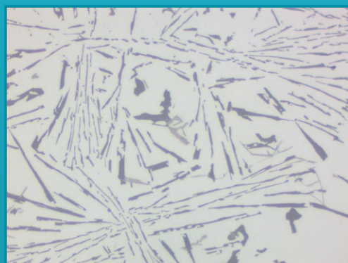
AISi, BF, 500x after polishing with Colloidal Silica, Alkaline, on Napal.
