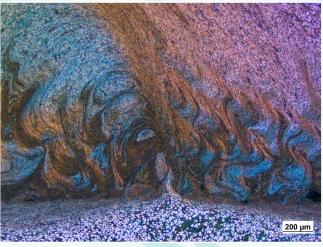
Aluminium friction stir weld, etched according to Barker, POL + Lambda Compensator, 50x
