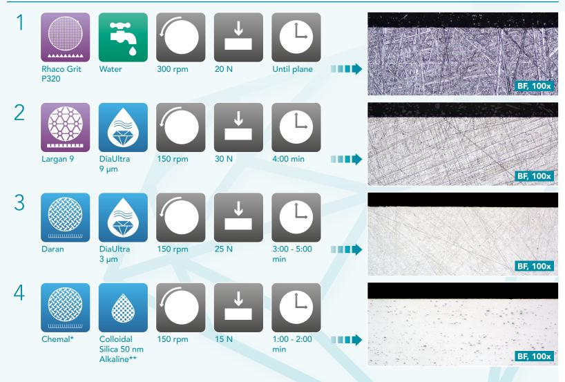
Times are stated for a 300 mm preparation system and forces for an individual 40 mm dia. sample.
