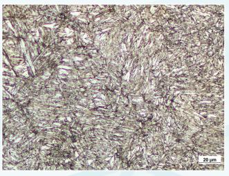
Tool Steel X40CrMoV51+QT, 410-470 HV, cross section etched with Nital 3%, BF, 500x
