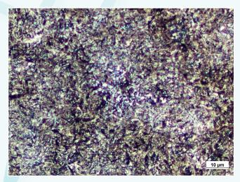
Tool Steel 100MnCrW4+QT, 700 HV, cross section etched with Nital 3%, BF, 1000x
