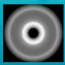
Graphic illustration showing the wear on a uniform grinding disc. White area shows the highest wear.
